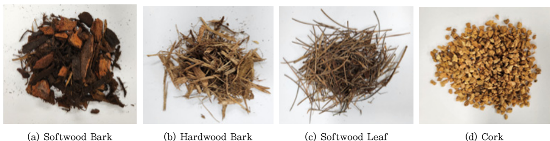
Fig. 1. Morphological properties of wood by-products.
