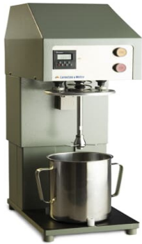
Fig. 1. TAPPI standard pulp disintegrator used for disintegration.
